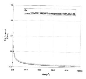
The close overlap of the increasing and decreasing shear sweeps demonstrates the pseudoplastic nature of this rheology modifier. A gap between the two curves would have indicated a longer viscosity recovery time, leaving a formulation prone to dripping when shear is removed.
